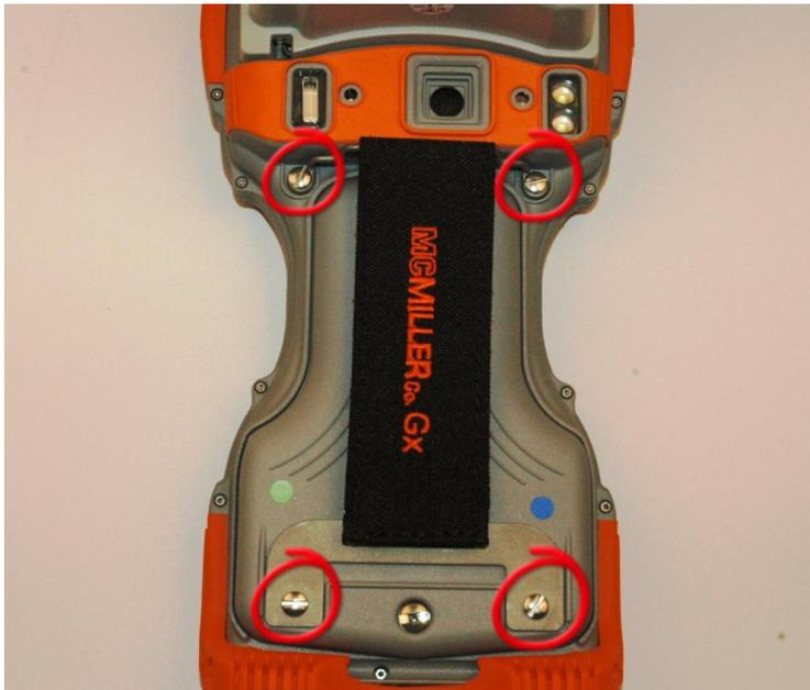
Next, remove the hand strap and associated brackets from the unit. This will reveal 4 tapped holes (two on the top and two on the bottom).
