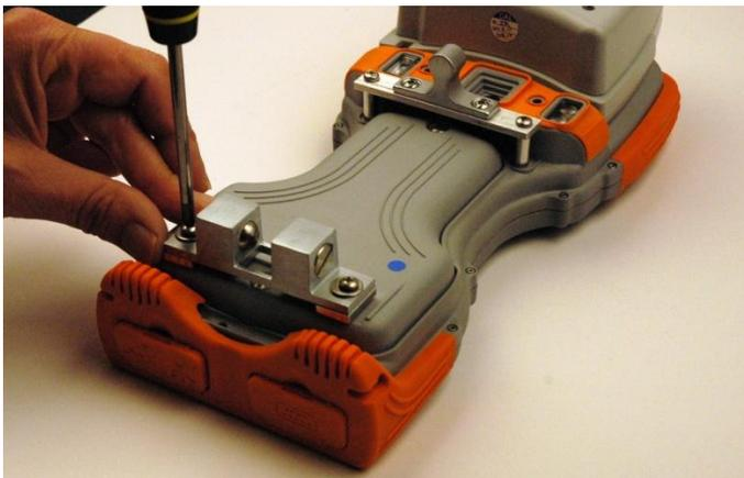
shown in the photograph opposite, and secure the Bottom Bracket using a Phillips-head screwdriver. **Note:** Do not over-tighten the screws so as not to strip the threads. Also, make sure that the flat washers are in place.
